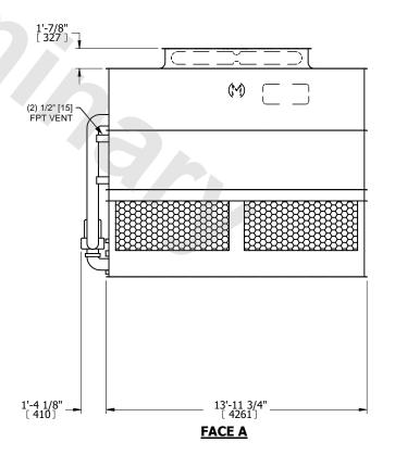
NO. OF SHIPPING SECTIONS **SHIPPING OPERATING** HEAVIEST SECTION 13330 lbs+ [6050] kg+ 20300 lbs+ [9210] kg+ 11320 lbs+ [5135] kg+ WEIGHT WEIGHT WEIGHT
