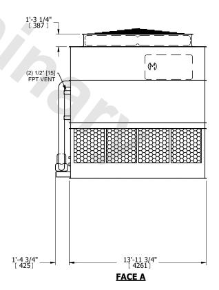
DRAWN BY: SLR NO. OF SHIPPING SECTIONS **SHIPPING** OPERATING HEAVIEST SECTION 18940 lbs+ [8595] kg+ 30010 lbs+ [13615] kg+ 15880 lbs+ [7205] kg+ WEIGHT WEIGHT WEIGHT
