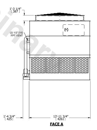
DRAWN BY: SLR NO. OF SHIPPING SECTIONS **SHIPPING** OPERATING HEAVIEST SECTION 19100 lbs+ [8665] kg+ 16040 lbs+ [7280] kg+ 30170 lbs+ [13685] kg+ WEIGHT WEIGHT WEIGHT
