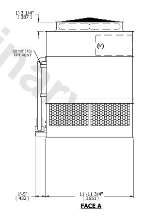
DRAWN BY: SLR NO. OF SHIPPING SECTIONS **SHIPPING** OPERATING HEAVIEST SECTION 18240 lbs+ [8275] kg+ 27720 lbs+ [12575] kg+ 15690 lbs+ [7120] kg+ WEIGHT WEIGHT WEIGHT
