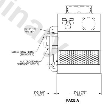
DRAWN BY: CAF NO. OF SHIPPING SECTIONS **SHIPPING** OPERATING HEAVIEST SECTION 2790 lbs+ [1270] kg+ 4310 lbs+ [1955] kg+ 2280 lbs+ [1035] kg+ WEIGHT WEIGHT WEIGHT
