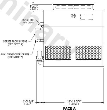
**SHIPPING** OPERATING HEAVIEST SECTION 11520 lbs+ [5230] kg+ 17520 lbs+ [7950] kg+ WEIGHT WEIGHT WEIGHT
