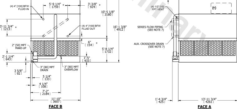
SHIPPING WEIGHT 24390 lbs+ [11065] kg+ OPERATING WEIGHT 37360 lbs+ [16950] kg+ HEAVIEST SECTION WEIGHT 21330 lbs+ [9680] kg+ NO. OF SHIPPING SECTIONS 2 DRAWN BY: JLG
