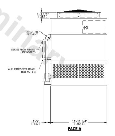
SHIPPING WEIGHT 20400 lbs+ [9255] kg+ OPERATING WEIGHT 30540 lbs+ [13855] kg+ HEAVIEST SECTION WEIGHT 17850 lbs+ [8100] kg+ NO. OF SHIPPING SECTIONS 2 DRAWN BY: TLM
