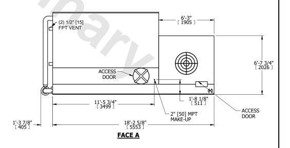
DRAWN BY: NO. OF SHIPPING SECTIONS **SHIPPING** OPERATING HEAVIEST SECTION 14980 lbs+ [6795] kg+ 14980 lbs+ [6795] kg+ 23410 lbs+ [10620] kg+ WEIGHT WEIGHT WEIGHT
