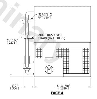
DRAWN BY: NO. OF SHIPPING SECTIONS **SHIPPING OPERATING** HEAVIEST SECTION 2720 lbs+ [1235] kg+ 1590 lbs+ [725] kg+ 3770 lbs+ [1715] kg+ WEIGHT WEIGHT WEIGHT
