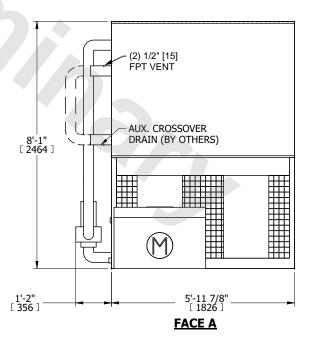
3070 lbs+ [1395] kg+ OPERATING WEIGHT 4230 lbs+ [1920] kg+ HEAVIEST SECTION WEIGHT 1940 lbs+ [880] kg+ NO. OF SHIPPING SECTIONS 2 DRAWN BY: TLS
