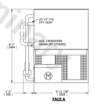
HEAVIEST SECTION 1940 lbs+ [880] kg+ NO. OF SHIPPING SECTIONS 2 DRAWN BY: TLS
