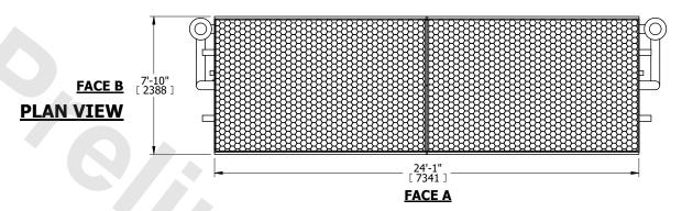
3'-8 7/8" \* (4) 4" [100] BFW FLUID IN (4) 1/2" [15] (4) 1/2" [15] FPT VENT **FPT VENT** 3'-11 3/4" \* [ 1213 ] (4) 4" [100] BFW 6'-1/2" [ 1842 ] FLUID OUT 13'-3 7/8" [ 4061 ] 2" [50] MPT MAKE-UP (2) ACCESS DOOR 7'-3 3/8" (2) 3" [80] MPT **ÖVERFLOW** 2'-11 7/8" [911] 3 1/8" [ 79 ] 10" [ 254 ] 1'-5" [ 432 ] 24'-1" [ 7341 ] 3'-2 5/8" [ 981 ] **FACE A** 3'-8 3/8" [ 1127 ] 2" [50] MPT DRAIN 7'-10" [ 2388 ]
