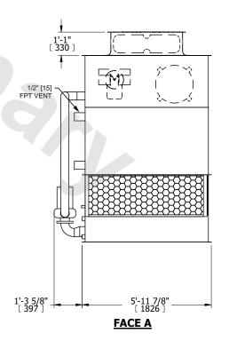
DRAWN BY: NO. OF SHIPPING SECTIONS **SHIPPING** OPERATING HEAVIEST SECTION 3730 lbs+ [1695] kg+ 5380 lbs+ [2445] kg+ 3220 lbs+ [1465] kg+ WEIGHT WEIGHT WEIGHT
