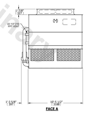
DRAWN BY: SLR NO. OF SHIPPING SECTIONS **SHIPPING OPERATING** HEAVIEST SECTION 9420 lbs+ [4275] kg+ 11060 lbs+ [5020] kg+ 15730 lbs+ [7140] kg+ WEIGHT WEIGHT WEIGHT
