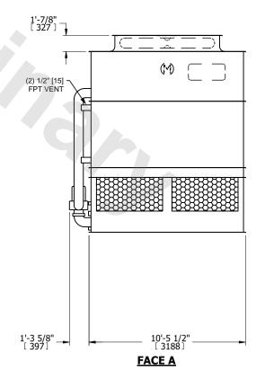
DRAWN BY: SLR NO. OF SHIPPING SECTIONS **SHIPPING OPERATING** HEAVIEST SECTION 16990 lbs+ [7710] kg+ 23130 lbs+ [10495] kg+ 15350 lbs+ [6965] kg+ WEIGHT WEIGHT WEIGHT
