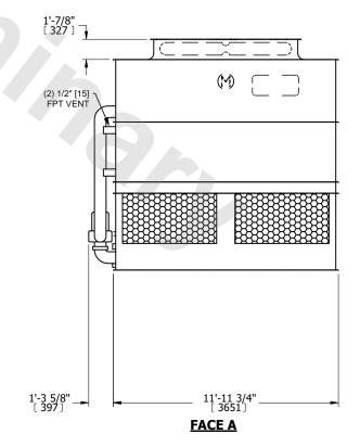
NO. OF SHIPPING SECTIONS **SHIPPING** OPERATING HEAVIEST SECTION 14220 lbs+ [6455] kg+ 20210 lbs+ [9170] kg+ 12350 lbs+ [5605] kg+ WEIGHT WEIGHT WEIGHT
