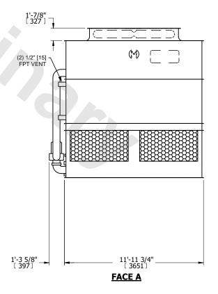
DRAWN BY: SLR NO. OF SHIPPING SECTIONS **SHIPPING OPERATING** HEAVIEST SECTION 14580 lbs+ [6615] kg+ 16450 lbs+ [7465] kg+ 23000 lbs+ [10435] kg+ WEIGHT WEIGHT WEIGHT
