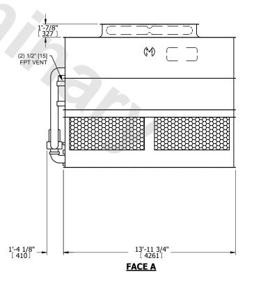
DRAWN BY: SLR NO. OF SHIPPING SECTIONS **SHIPPING OPERATING** HEAVIEST SECTION 13700 lbs+ [6215] kg+ 20000 lbs+ [9075] kg+ 11620 lbs+ [5275] kg+ WEIGHT WEIGHT WEIGHT
