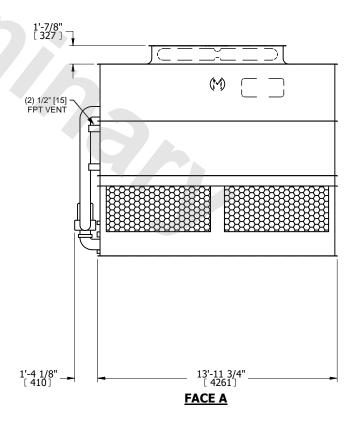
DRAWN BY: SLR NO. OF SHIPPING SECTIONS **SHIPPING** OPERATING HEAVIEST SECTION 16250 lbs+ [7375] kg+ 14170 lbs+ [6430] kg+ 23220 lbs+ [10535] kg+ WEIGHT WEIGHT WEIGHT
