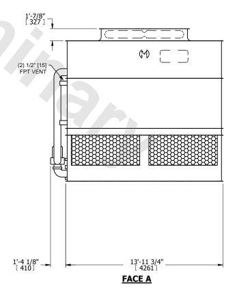
NO. OF SHIPPING SECTIONS **SHIPPING** OPERATING HEAVIEST SECTION 19370 lbs+ [8790] kg+ 21450 lbs+ [9730] kg+ 29720 lbs+ [13485] kg+ WEIGHT WEIGHT WEIGHT
