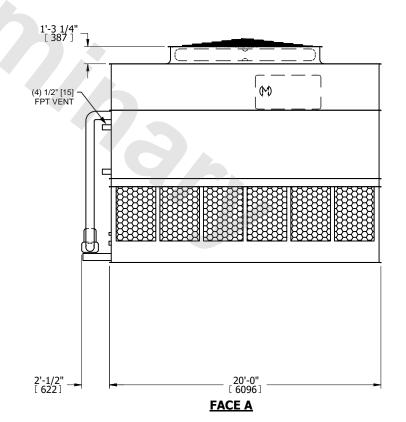
DRAWN BY: SLR NO. OF SHIPPING SECTIONS **SHIPPING** OPERATING HEAVIEST SECTION 32770 lbs+ [14865] kg+ 37280 lbs+ [16910] kg+ 54490 lbs+ [24720] kg+ WEIGHT WEIGHT WEIGHT
