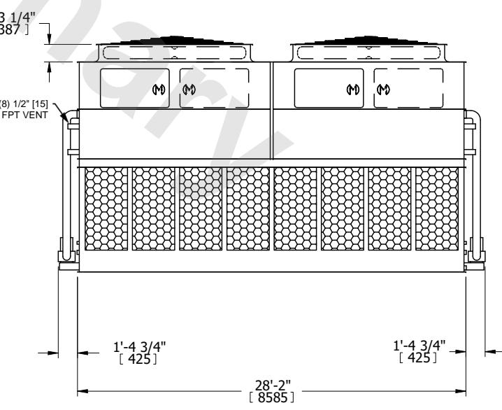
SHIPPING WEIGHT 78600 lbs+ [35655] kg+ OPERATING WEIGHT 119060 lbs+ [54005] kg+ HEAVIEST SECTION WEIGHT 16540 lbs+ [7505] kg+ NO. OF SHIPPING SECTIONS 6 DRAWN BY: SLR
