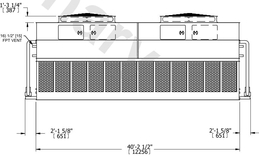
SHIPPING WEIGHT 107780 lbs+ [48890] kg+ OPERATING WEIGHT 165840 lbs+ [75225] kg+ HEAVIEST SECTION WEIGHT 22410 lbs+ [10170] kg+ NO. OF SHIPPING SECTIONS 6 DRAWN BY: SLR
