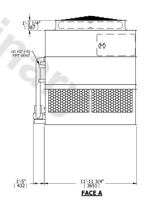
DRAWN BY: SLR NO. OF SHIPPING SECTIONS **SHIPPING OPERATING** HEAVIEST SECTION 12260 lbs+ [5565] kg+ 14810 lbs+ [6720] kg+ 22320 lbs+ [10125] kg+ WEIGHT WEIGHT WEIGHT
