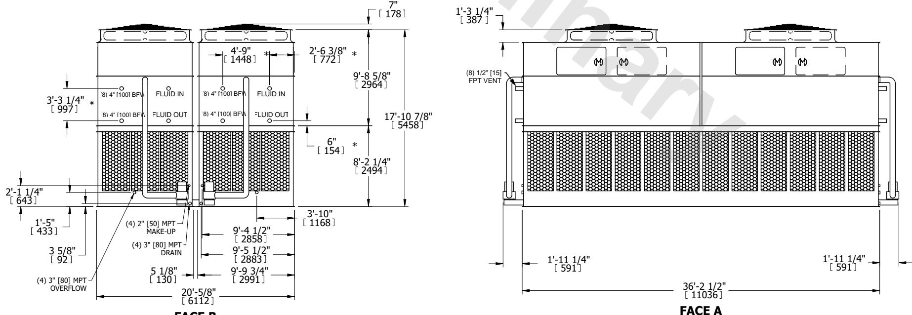
SHIPPING WEIGHT 116040 lbs+ [52635] kg+ OPERATING WEIGHT 169400 lbs+ [76840] kg+ HEAVIEST SECTION WEIGHT 25190 lbs+ [11430] kg+ NO. OF SHIPPING SECTIONS 6 DRAWN BY: SLR
