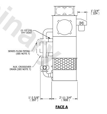
DRAWN BY: NO. OF SHIPPING SECTIONS **SHIPPING** OPERATING HEAVIEST SECTION 1470 lbs+ [670] kg+ 2050 lbs+ [930] kg+ 1190 lbs+ [540] kg+ WEIGHT WEIGHT WEIGHT
