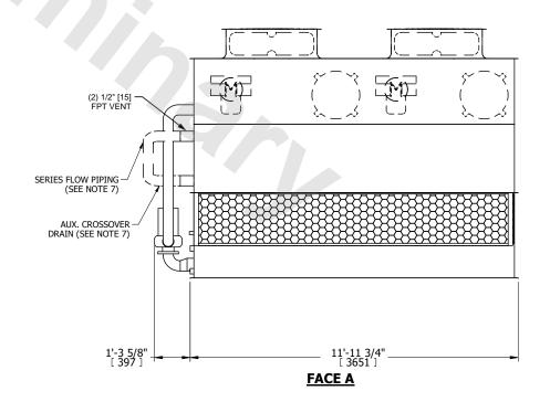
DRAWN BY: **SHIPPING** OPERATING HEAVIEST SECTION NO. OF SHIPPING SECTIONS 5840 lbs+ [2650] kg+ 8740 lbs+ [3965] kg+ 5020 lbs+ [2280] kg+ WEIGHT WEIGHT WEIGHT
