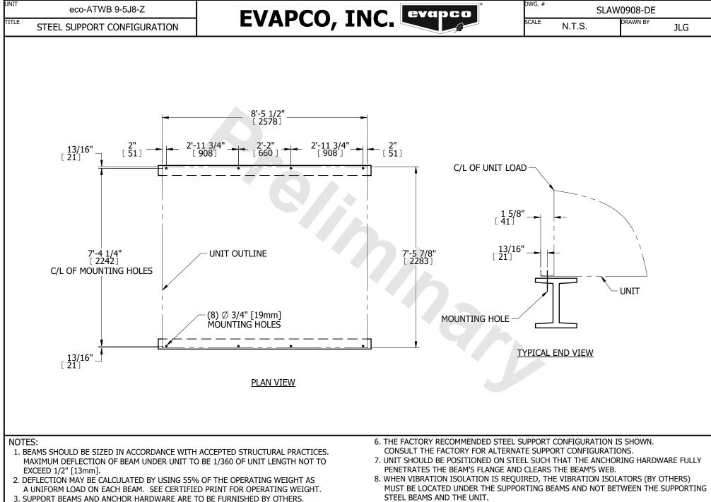
ANCHOR HARDWARE TO BE ASTM A325 5/8" [16mm] BOLT OR EQUIVALENT.
