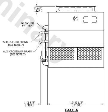
DRAWN BY: JLG NO. OF SHIPPING SECTIONS **SHIPPING** OPERATING HEAVIEST SECTION 10940 lbs+ [4965] kg+ 15610 lbs+ [7085] kg+ 9300 lbs+ [4220] kg+ WEIGHT WEIGHT WEIGHT
