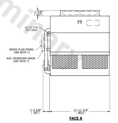
DRAWN BY: JLG NO. OF SHIPPING SECTIONS **SHIPPING** OPERATING HEAVIEST SECTION 16390 lbs+ [7435] kg+ 22940 lbs+ [10410] kg+ 14520 lbs+ [6590] kg+ WEIGHT WEIGHT WEIGHT
