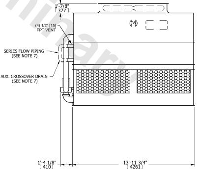
SHIPPING WEIGHT 13700 lbs+ [6215] kg+ OPERATING WEIGHT 20000 lbs+ [9075] kg+ HEAVIEST SECTION WEIGHT
