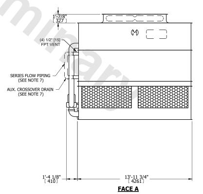
NO. OF SHIPPING SECTIONS **SHIPPING** OPERATING HEAVIEST SECTION 18840 lbs+ [8550] kg+ 26460 lbs+ [12005] kg+ 16760 lbs+ [7605] kg+ WEIGHT WEIGHT WEIGHT
