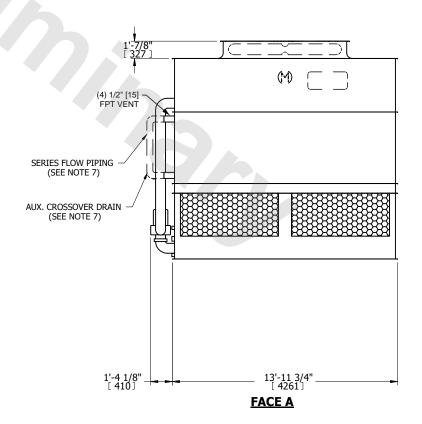
DRAWN BY: JLG NO. OF SHIPPING SECTIONS **SHIPPING OPERATING** HEAVIEST SECTION 19370 lbs+ [8790] kg+ 21450 lbs+ [9730] kg+ 29720 lbs+ [13485] kg+ WEIGHT WEIGHT WEIGHT
