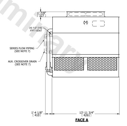
DRAWN BY: JLG **SHIPPING** OPERATING HEAVIEST SECTION NO. OF SHIPPING SECTIONS 21450 lbs+ [9730] kg+ 29720 lbs+ [13485] kg+ 19370 lbs+ [8790] kg+ WEIGHT WEIGHT WEIGHT
