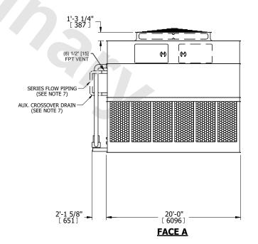
SHIPPING WEIGHT 75300 lbs+ [34160] kg+ OPERATING WEIGHT 109720 lbs+ [49770] kg+ HEAVIEST SECTION WEIGHT 33140 lbs+ [15035] kg+ NO. OF SHIPPING SECTIONS 4 DRAWN BY: JLG
