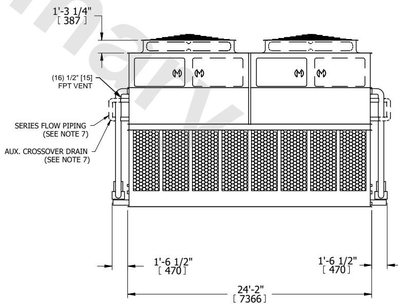
SHIPPING WEIGHT 68700 lbs+ [31165] kg+ OPERATING WEIGHT 103200 lbs+ [46815] kg+ HEAVIEST SECTION WEIGHT 14380 lbs+ [6525] kg+ NO. OF SHIPPING SECTIONS 6 DRAWN BY: **JLG**
