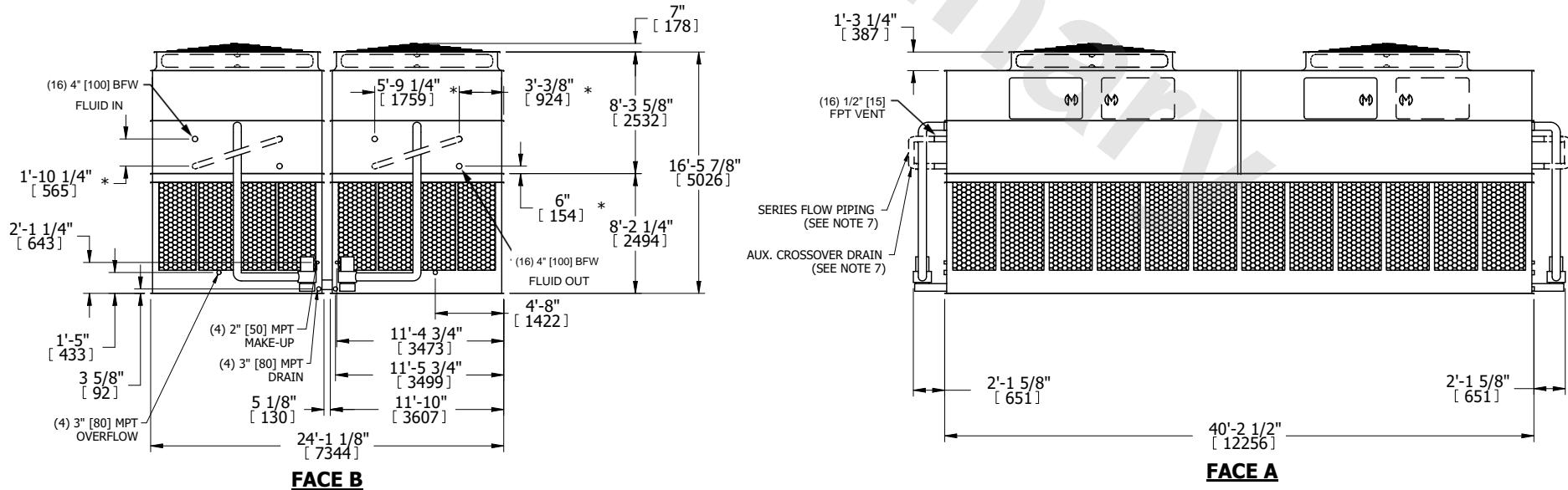
SHIPPING WEIGHT 107780 lbs+ [48890] kg+ OPERATING WEIGHT 165840 lbs+ [75225] kg+ HEAVIEST SECTION WEIGHT 22410 lbs+ [10170] kg+ NO. OF SHIPPING SECTIONS 6 DRAWN BY: JLG
