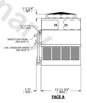
SHIPPING WEIGHT 34780 | lbs+ [15780] kg+ | OPERATING WEIGHT 51100 | lbs+ [23180] kg+ | HEAVIEST SECTION WEIGHT 14830 | lbs+ [6730] kg+ | NO. OF SHIPPING SECTIONS 4 | DRAWN BY: SLR
