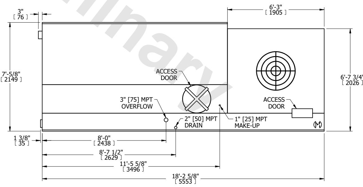
SHIPPING WEIGHT 3450 lbs+ [1565] kg+ OPERATING WEIGHT 7010 lbs+ [3180] kg+ HEAVIEST SECTION WEIGHT 3450 lbs+ [1565] kg+ NO. OF SHIPPING SECTIONS 1 DRAWN BY: JLG
