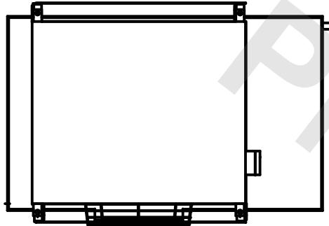
Technical drawing of a unit with a fan and a drain. The top horizontal dimension is 67 3/8. The left vertical dimension is 6 1/4. The right vertical dimension is 19 1/8. The center horizontal dimension is 42. The bottom horizontal dimension is 42. The bottom vertical dimension is 6 1/4. A 1" MPT DRAIN is shown at the bottom right.
