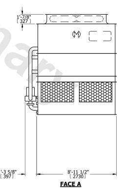
DRAWN BY: SLR NO. OF SHIPPING SECTIONS **SHIPPING OPERATING** HEAVIEST SECTION 8020 lbs+ [3640] kg+ 9460 lbs+ [4295] kg+ 12390 lbs+ [5625] kg+ WEIGHT WEIGHT WEIGHT
