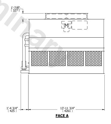
DRAWN BY: JLG NO. OF SHIPPING SECTIONS **SHIPPING OPERATING** HEAVIEST SECTION 10970 lbs+ [4980] kg+ 15520 lbs+ [7040] kg+ 8890 lbs+ [4035] kg+ WEIGHT WEIGHT WEIGHT
