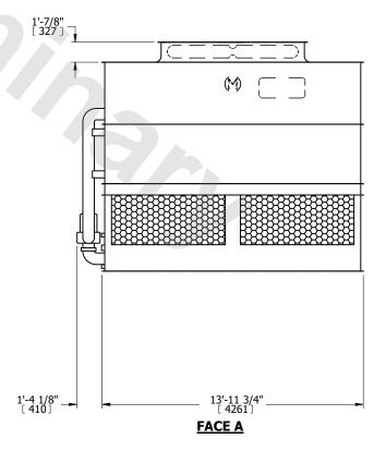
DRAWN BY: SLR NO. OF SHIPPING SECTIONS **SHIPPING** OPERATING HEAVIEST SECTION 16030 lbs+ [7275] kg+ 20870 lbs+ [9470] kg+ 13950 lbs+ [6330] kg+ WEIGHT WEIGHT WEIGHT
