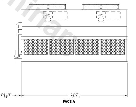
SHIPPING WEIGHT 16990 lbs+ [7710] kg+ OPERATING WEIGHT 23990 lbs+ [10885] kg+ HEAVIEST SECTION WEIGHT 13890 lbs+ [6305] kg+ NO. OF SHIPPING SECTIONS 2 DRAWN BY: JLG
