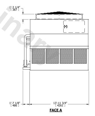
SHIPPING WEIGHT 15740 lbs+ [7140] kg+ OPERATING WEIGHT 23310 lbs+ [10575] kg+ HEAVIEST SECTION WEIGHT 12680 lbs+ [5755] kg+ NO. OF SHIPPING SECTIONS 2 DRAWN BY: TLM
