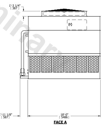
DRAWN BY: SLR NO. OF SHIPPING SECTIONS **SHIPPING** OPERATING HEAVIEST SECTION 38550 lbs+ [17490] kg+ 34630 lbs+ [15710] kg+ 49350 lbs+ [22385] kg+ WEIGHT WEIGHT WEIGHT
