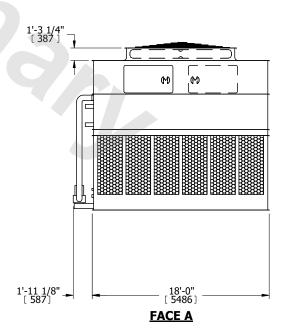
NO. OF SHIPPING SECTIONS **SHIPPING** OPERATING HEAVIEST SECTION 16260 lbs+ [7380] kg+ 38640 lbs+ [17530] kg+ 54220 lbs+ [24595] kg+ WEIGHT WEIGHT WEIGHT
