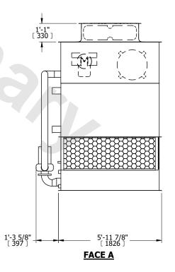
NO. OF SHIPPING SECTIONS **SHIPPING** OPERATING HEAVIEST SECTION 3740 lbs+ [1700] kg+ 3230 lbs+ [1470] kg+ 4890 lbs+ [2220] kg+ WEIGHT WEIGHT WEIGHT
