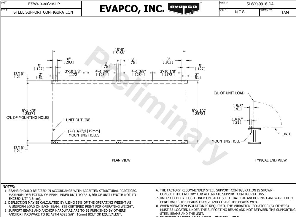
BEAMS MUST BE LOCATED UNDER THE FULL LENGTH OF THE PAN SECTION.
